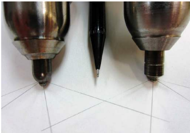
Close up of nozzle end of two injectors. Lines indicate the spray path.
