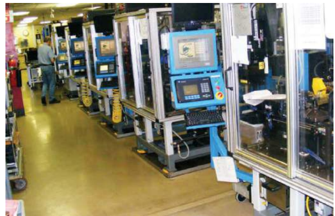
High-production automatic microhole EDM machines run untended for eight hours at a major manufacturing facility.
